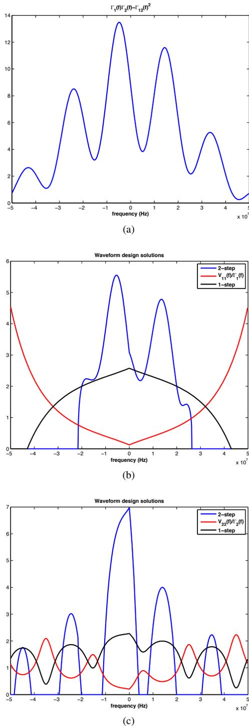
Fig. 4. Results for example-2 criteria for waterfiling (red), waterfilling solution (black), and two step MI solution (blue) are shown, and (a)  $\Gamma_1(f)\Gamma_2(f) - \Gamma_{12}^2(f)$ , b)  $|S_1(f)|^2$  c)  $|S_2(f)|^2$
