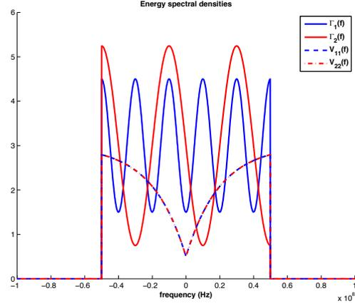
Fig. 1. Noise PSDs and target impulse response ESVs for Example -1
